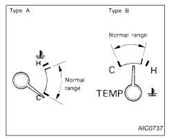
The gauge indicates the engine coolant temperature.
