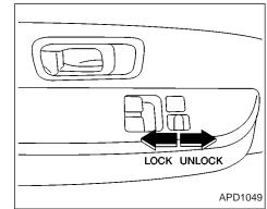
To lock from the outside without a key, push the door lock button (driver side only) or the door lock knob (driver or passenger side), then close the door. When locking the door this way, be certain not to leave the key inside the vehicle. If the key is left in the ignition, all doors will unlock automatically.
