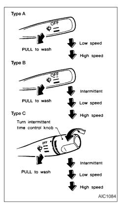
The ignition switch must be in the ON position for the wipers or washer to be activated. Push the lever down to operate the wipers, and pull the lever toward you to operate the washer. Operating the washer automatically cycles the wipers several times.
