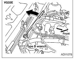
2. Remove spark plugs with a spark plug wrench, (type A or B) supplied in the vehicle's tool bag.
