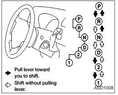
Shifting with automatic transmission (KA24DE engine)
