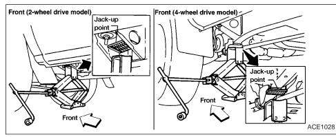
Jacking up the vehicle and removing the wheel
