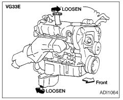
5. Remove the drain plug with a wrench and completely drain the oil.
