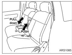
Pull down the armrest/storage compartment. Push the release button and lift the armrest assembly to the upright position to access the storage compartment and cup holder.
