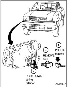
The headlight is a semi-sealed beam type which uses a replaceable headlight (halogen) bulb.
