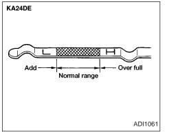
Remove the dipstick again and check the oil level. It should be between the H (High) and L (Low) marks. If the oil level is below the L (Low) mark, remove the oil filler cap and pour recommended oil through the opening. Do not overfill.
