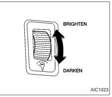
The instrument brightness control operates when the light switch is in the EDdE or EO position.
