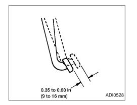
Press the pedal by hand and be sure the free travel is within the above limit. If free travel is out of the range shown above, see an authorized NISSAN dealer.
