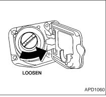
The fuel filler cap is a screw-on ratcheting type. Tighten the cap clockwise until ratcheting clicks are heard.
