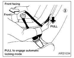
Pull on the shoulder belt until all of the belt is fully extended. At this time, the retractor is in the automatic locking mode (child restraint mode). It reverts back to emergency locking mode when the belt is fully retracted.
