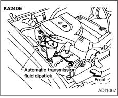
after the engine is warmed up and before driving. However, the fluid should be re-checked using the HOT range.
