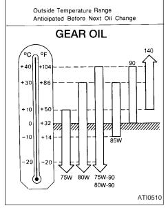
80W-90 for the differential and 75W-90 for the transfer case are preferable for ambient temperatures below 104°F (40°C).
