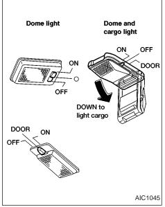
Each dome light has a three-position switch and operates regardless of ignition key position.
