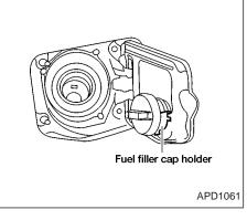
Put the fuel filler cap on the cap holder while refueling.
