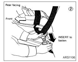
Route the seat belt tongue through the child restraint and insert the belt tongue into the buckle until you hear and feel the latch engage. Be sure to follow the child restraint manufacturer's instructions for belt routing.
