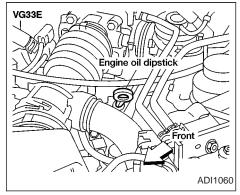
4. Remove the dipstick and wipe it clean. Reinsert it all the way.
