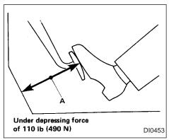
With the engine running, check distance A between the upper surface of the pedal and the metal floor.
