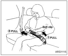
2. Tighten the belt by pulling the free end of the belt away from the tongue, then pull the belt clip to take up the slack.
