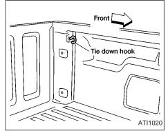
For your convenience, tie down hooks are placed at each corner of the truck box. These may be used to help secure cargo loaded into the truck box.
