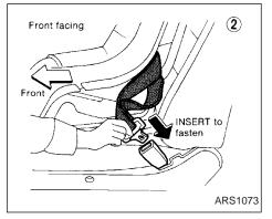
2. Route the seat belt tongue through the child restraint and insert the belt tongue into the buckle until you hear and feel the latch engage. Be sure to follow the child restraint manufacturer's instructions for belt routing.
