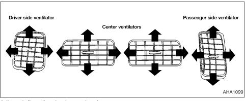
Adjust air flow direction by moving the ventilators slides and ventilator assemblies.
