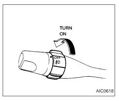
To turn the front fog lights on, rotate the switch to the  $\ddagger$  position.
