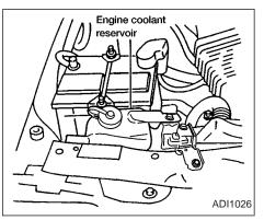
CHECKING ENGINE COOLANT LEVEL
