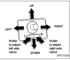
Push the right or left side of the switch to adjust the right or left side mirror, then control the lever.
