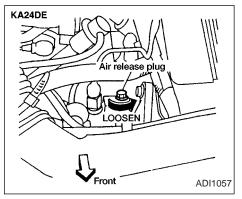
10. Open and close the air release plug to release air. Then fill the radiator again and install the radiator cap.
