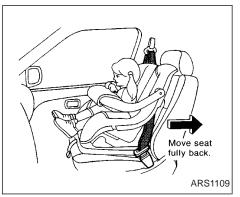
FRONT FACING INSTALLATION ON FRONT PASSENGER SEAT (Three-point type with retractor)
