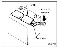
1. Gently pry between the battery cap and cover as illustrated to remove the cap.
