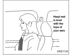
Adjust the top of the head restraint even with the tops of your ears.
