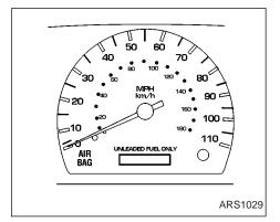
The supplemental air bag warning light, displaying  $B_{AG}^{AIR}$  in the instrument panel, monitors the circuits of the supplemental air bag system. The circuits monitored by the supplemental air bag warning light are the diagnosis sensor unit, the supplemental air bag modules and all related wiring.
