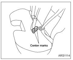
TWO-POINT TYPE WITHOUT RETRACTOR (Jump seat and center of bench seat)
