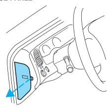
To remove a fuse, use the fuse puller provided on the fuse panel cover.
