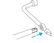
6. Remove the spare tire security lock and cable.
